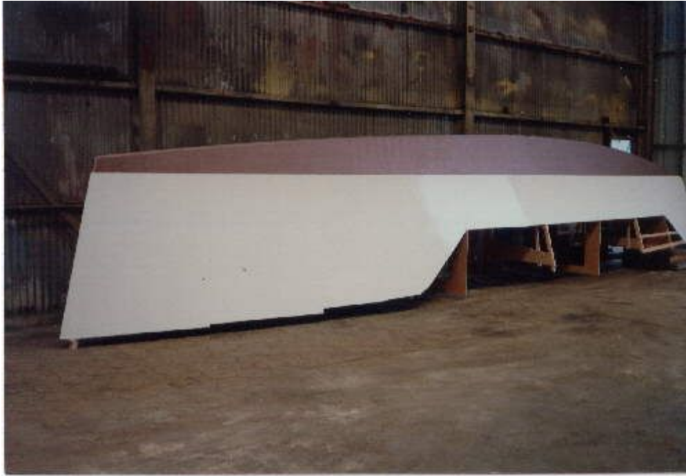
Hull ready for turning
